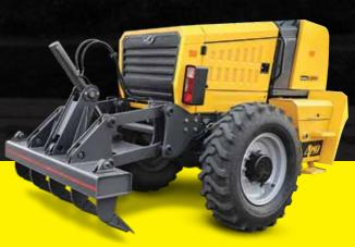
**Optional Attachment:** The RoadMaster G9075 comes with the option of having additional ripper fitments for added versatility. The Ripper is perfect for ripping hard compacted surfaces before grading.
