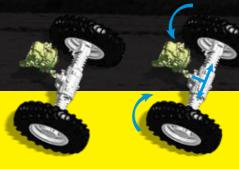
100% Mechanical Differential Lock helps in higher power generation and equal distribution of motion in the rear tyres. Ensures better performance in grading and is useful on muddy, marshy soils. The machine does not get stuck anywhere.
