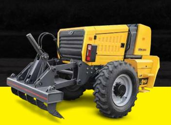
**Optional Attachment:** The RoadMaster G9075 comes with the option of having additional ripper fitments for added versatility. The Ripper is perfect for ripping hard compacted surfaces before grading.
